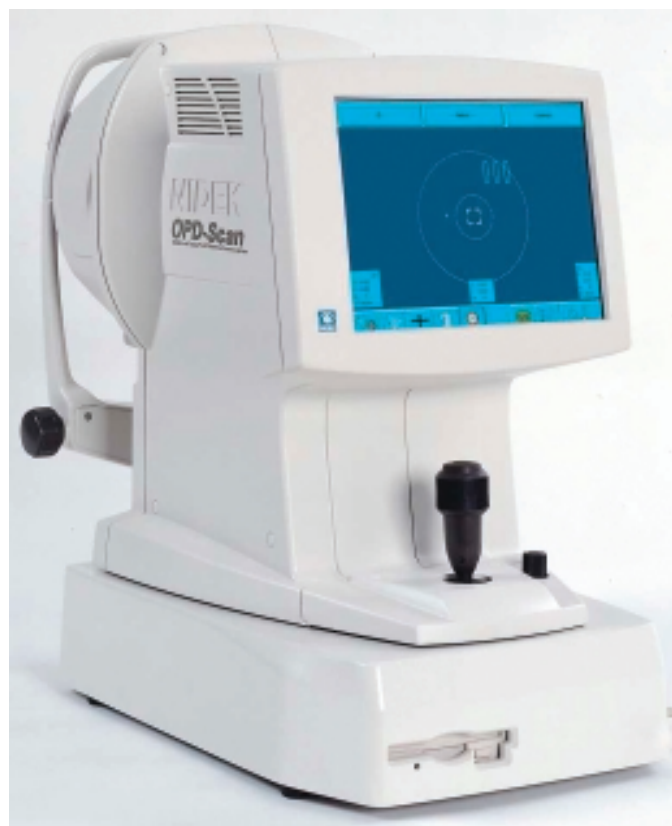
Figure 1: OPD-Scan topographer and aberrometer in the same device, used to measure corneal and entire eye aberrations.
